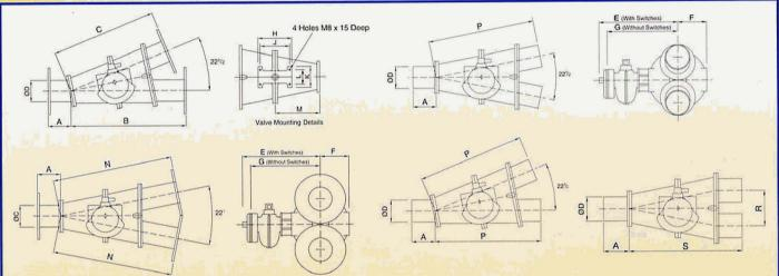
PC Diverters with Flange Connections PC Diverters with Plain Tube Spigots
